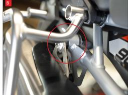
A) Start by loosening the clamp on the original exhaust.
